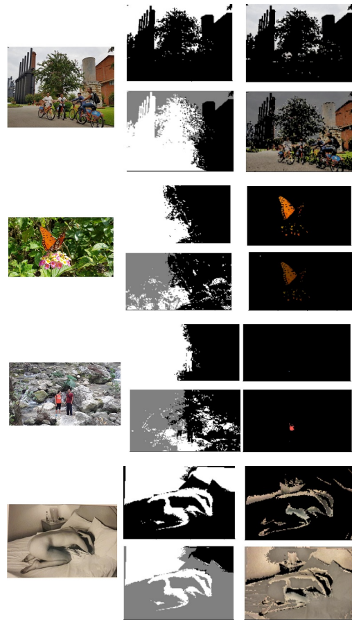
Fig. 4. Results of the segmentation of images 6 to 10, original image (left), segmentation obtained using the eigenvector associated with the second smallest eigenvalue in grayscale and RGB (center and right above) and segmentation obtained using the associated eigenvectors to the second and third eigenvalue smaller in gray scale and RGB (center and right below).
