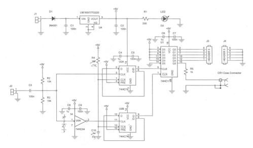
Figure 3: Ground bounce circuit schematic.
