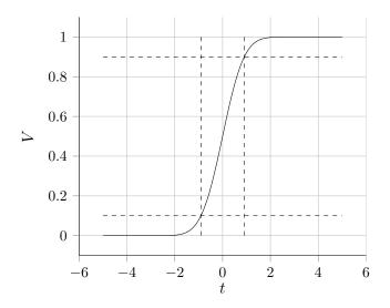
Figure 1: Gaussian edge with a 10-90 rise marked
