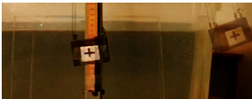
Figure 16: Two frames layered on top of each other, one showing the pendulum in the equilibrium position and the other showing it at maximum y-displacement.
