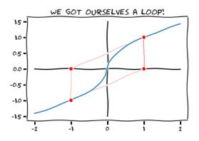
FIGURE 3.3. Newton-Raphson fails for some functions
