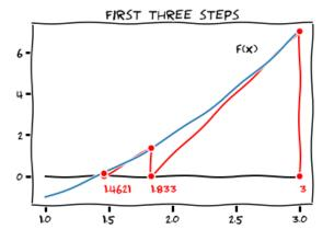
FIGURE 3.1. Newton-Raphson iterative method
