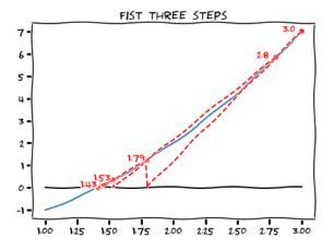
FIGURE 3.5. Secant iterative method
